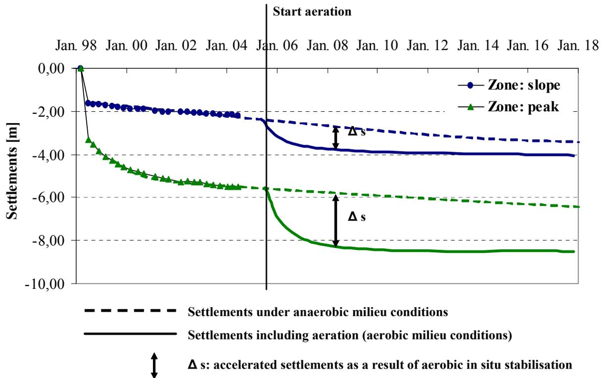
Figure 2: Course of the settlements in the proximity of two gas wells in the peak and slope area under anaerobic and aerobic milieu conditions
