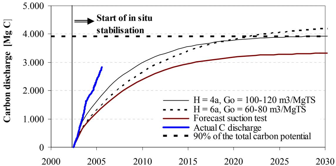
Figure 4: Range of the biologically convertible carbon, dischargeable via the gas path, under anaerobic milieu conditions from 2002 onwards. Comparison with the actual carbon discharge as a result of aerobic in situ stabilisation
