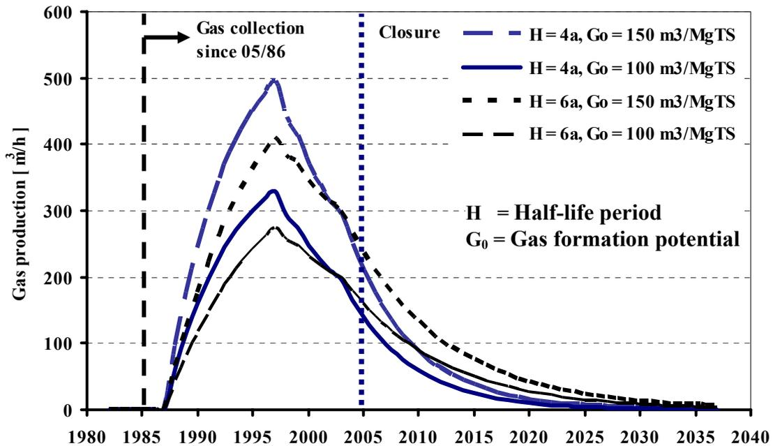
Figure 1: Range of the potential landfill gas production of a landfill section of a TASI II landfill which was filled up until 1996, including variation of the half-life period and of the carbon content
